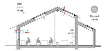
In the event of rain and high CO<sub>2</sub> levels, fresh air is supplied through the flaps in upper part of roof windows or additional mechanical ventilation if needed.
