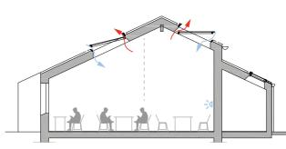
CO<sub>2</sub> sensors control the air quality in the classroom. The roof windows open automatically and close again when minimum CO<sub>2</sub> setpoint is achieved or if it rains.
