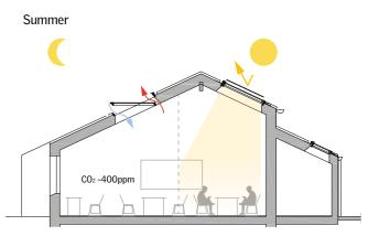
In summer, automatically controled exterior sunscreening helps to control solar heat gains. While manual control of interior blinds provides the possibility of adjusting daylight levels according to the need of teacher and pupils.
