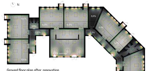
Ground floor plan after renovation daylight factor results
