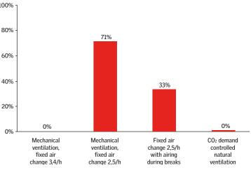
The comparison of the results shows that demand-controlled natural ventilation with CO<sub>2</sub> sensors provides much better air quality to the room than the fixed air change of 2.5 (calculated according to BR 2010). Demand-controlled natural ventilation is operated by CO<sub>2</sub> sensors installed in each classroom. The opening of the windows is controlled by two setpoints:
