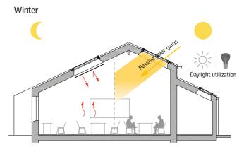
Automatically controlled interior sunscreening help to minimise heat losses at night during winter.
